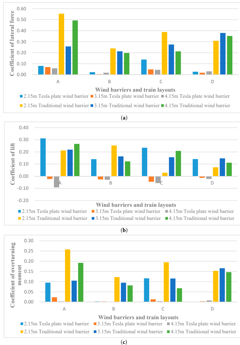
Figure 22: Diagram of three force components on the train. (a) Coefficient of lateral force; (b) Coefficient of lift force; (c) Coefficient of overturning moment.
