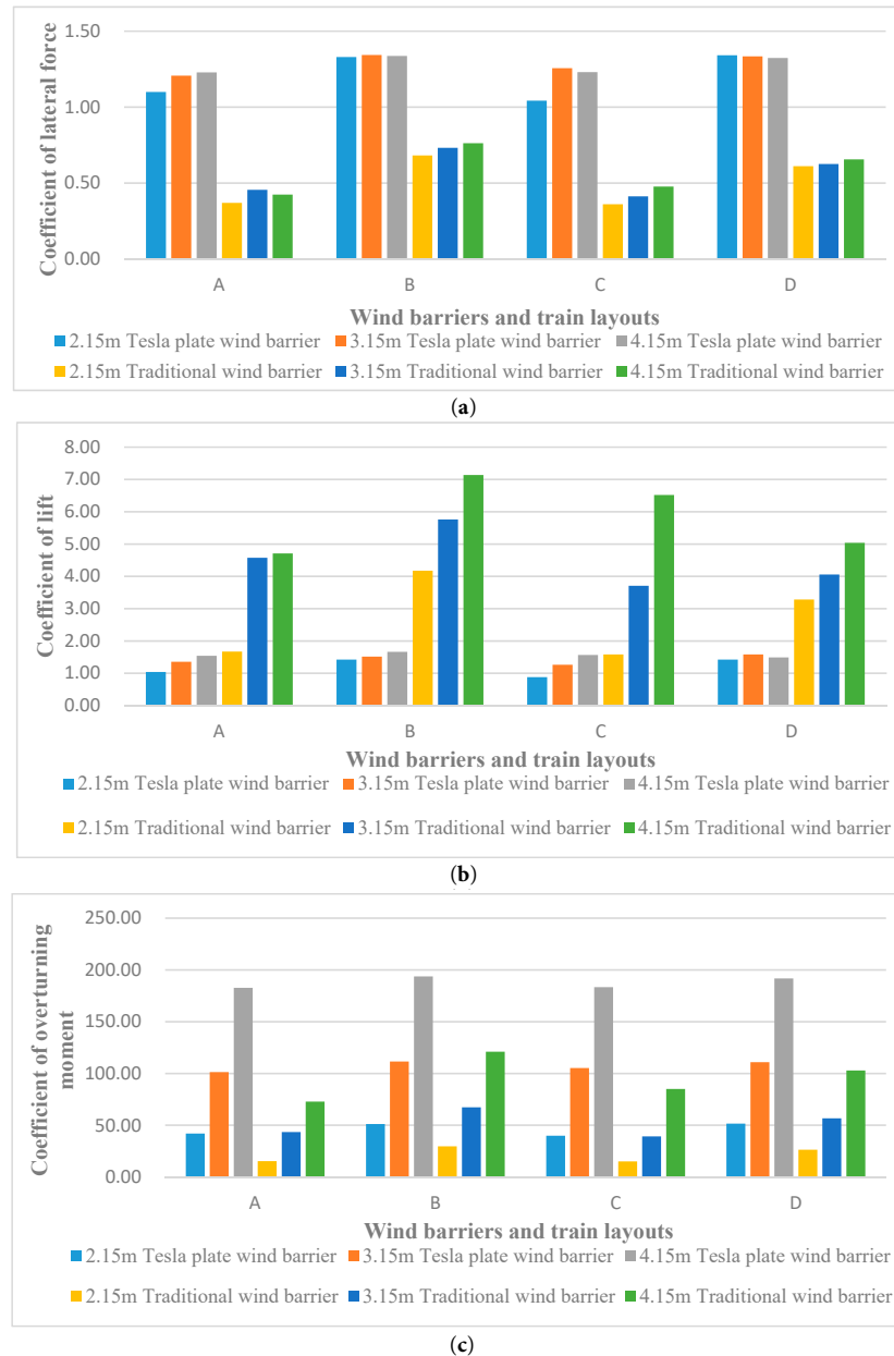
Figure 23: Diagram of three force components on the upstream wind barrier. (a) Coefficient of lateral force; (b) Coefficient of lift force; (c) Coefficient of overturning moment.
